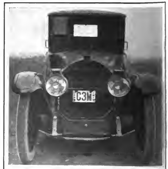
To aid in making the Locomobile lower the front axle sweeps in a continuous curve between the steering knuckles instead of dropping abruptly
